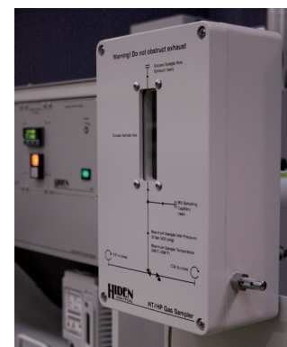
HT/HP inlet (up to 30 bar at 200°C)
