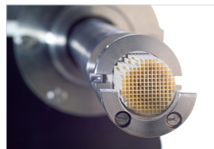
Intra-catalyst sampling of gas and temperature
