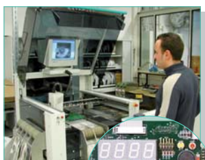
Pick & place assembly station (SMD)
